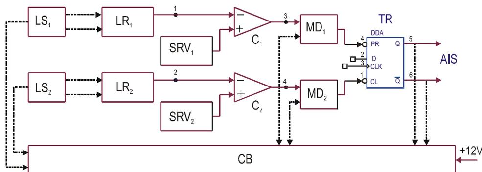
Fig.3. Structural scheme of the device for counting of bottles
