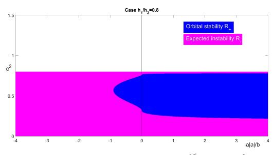
**Figure 3.** The region of orbital stability (d'' > 0) for  $h_1/h_2 = 0.8$ ,  $\frac{a|a|}{b} \in (-4, 4)$  and  $c^2 \in (0, 0.8)$ : **left half-plane** is for a < 0; **right half-plane** is for a > 0.
