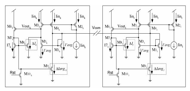
Figure 3. Cells 1 and k (out of N) of the LTA circuit.
