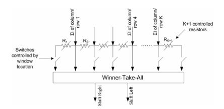
Figure 4. The X-COM and Y-COM update circuit implementation
