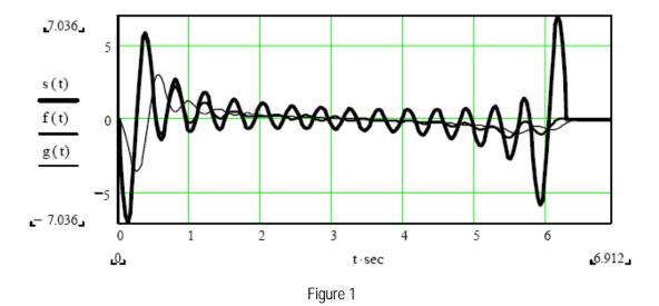
At the figure 1 here are three curves: the first one, which is marked as s(t), is model of sounding signal. The second one (f(t)) is misshaped signal by random frequency fluctuation, the third one (g(t)) is misshaped
