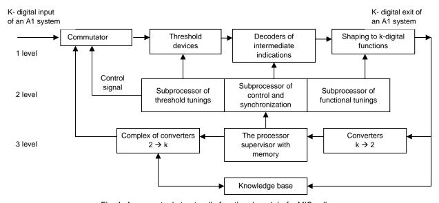
Fig. 1. A conceptual structurally functional model of a MIS cell.
