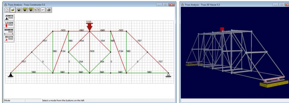
Fig. 5. Elica Truss Analysis applications
