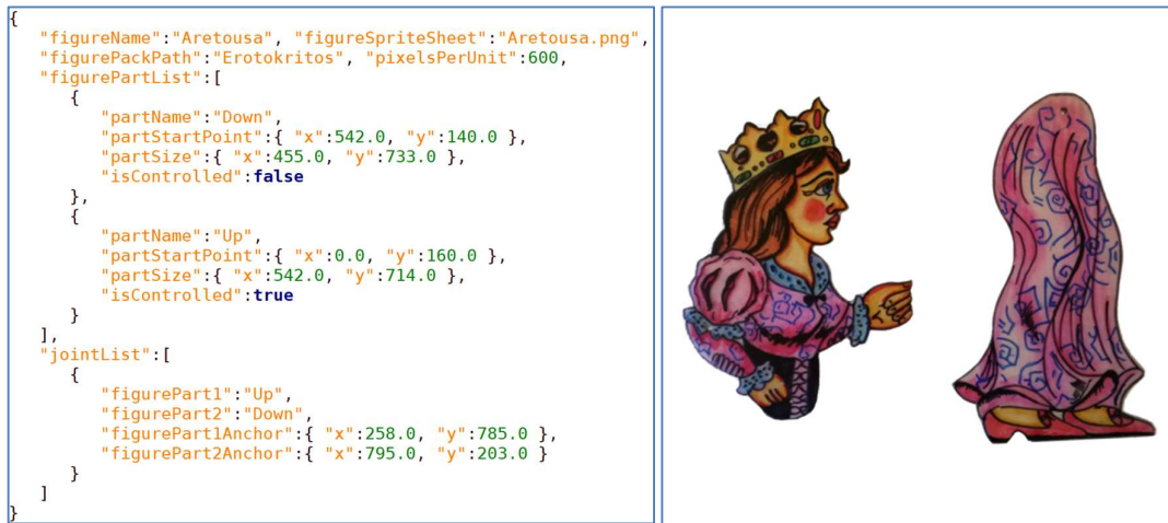
Figure 30: Digital puppet representation. On the left, the json file describing how the puppet is composed of different parts, where these parts can be found in the corresponding sprite sheet and where the joint anchors are placed. On the right, the corresponding sprite sheet is depicted.
