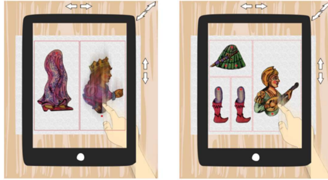
Figure 28: Digitization of shadow theatre puppets using ePuppet. The parts of the puppet are put on a flat surface with a constant color background (e.g., on a sheet of paper). The parts and the mobile device are moved as needed so that the parts are framed within the red boundaries shown in screen overlay and the joint anchors (red circles) are positioned correctly. Then, a photograph is taken that is transformed by ePuppet into a correct digital puppet representation.
