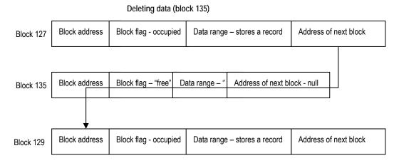
Fig. 2 Deleting data in block structures
