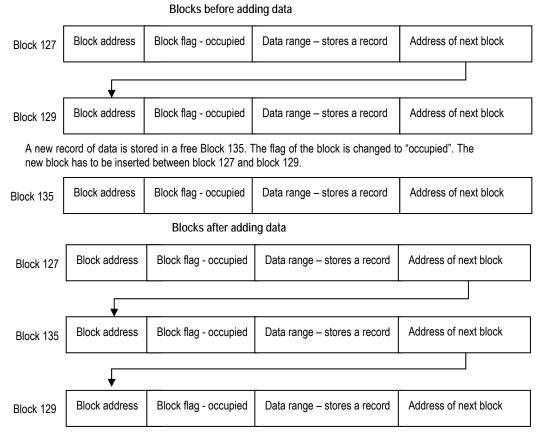
Fig. 1. Adding data in block structures
